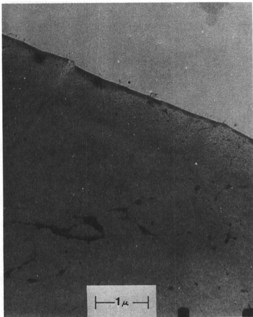
FIGURE 12 Electron photomicrograph cross-sections of the air-dried surface region of a Polymer I membrane coagulated at 0° C
