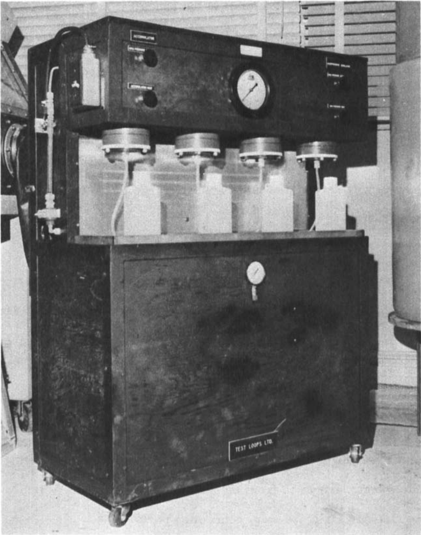
FIGURE 2 PVC Reverse Osmosis Test Unit
