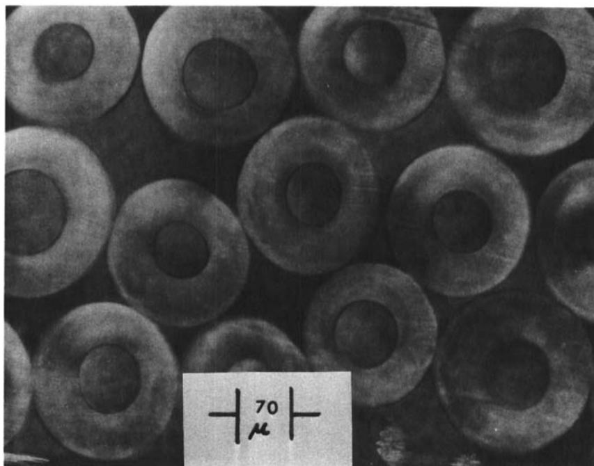
FIGURE 28 Photomicrograph of dry-spun Polymer I hollow fibers (Sample A)
