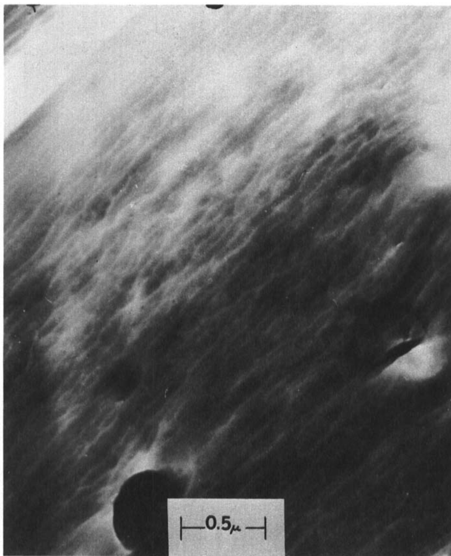
FIGURE 33 Electron photomicrograph of the interior region of a Polymer I hollow fiber
